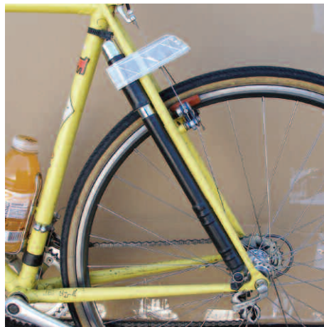
Robert - Problem: He shoulders his bike a lot in cyclo-cross and taking the bike up long flights of stairs. The pump inside the main triangle would get in the way, would get pushed out.
