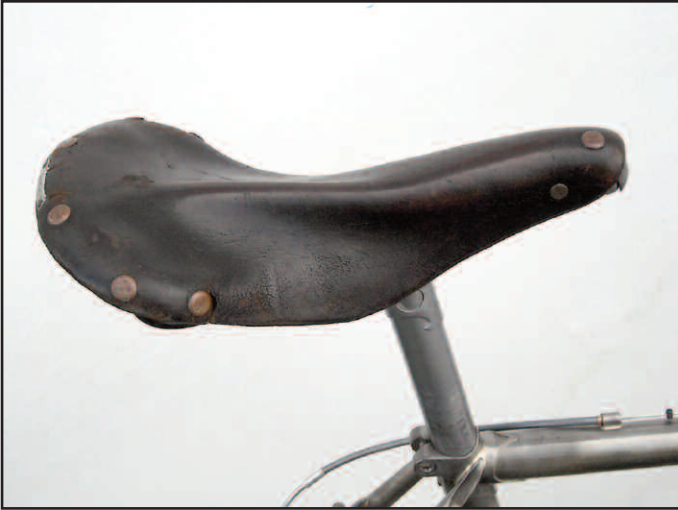
This old Ideale saddle was the most swaybacked, ridge-y saddle of all time. Fixed with fine firm foam, it's comfortable. Ideally, no pun intended, the leather would be soaked and softened, then stuffed. The foam would prevent further sagging...as foam does.
