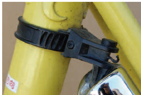
Solution: A pump clip mounted to the seat tube. The business end of the pump nests in the crook of the chainstay-seatstay-dropout. It holds fast.
