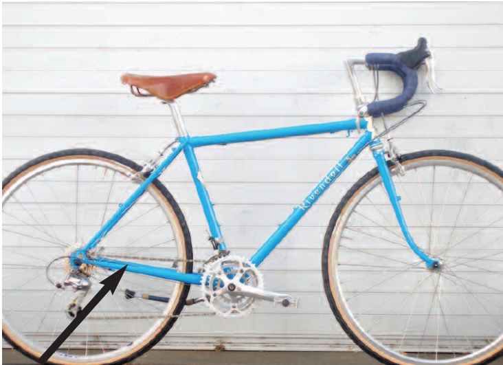
This chainstay is 45.5cm long, longer than the chainstays on most touring bikes, even biggies. The frame, coincidentally, is also 45.5cm. And the bike handles incredibly. Brisky-frisky, no twitchiness, just great.
