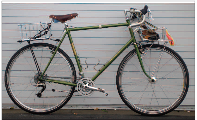
My pbh is 85 and the frame is a 60, and the top tube slopes up 6-degrees.
