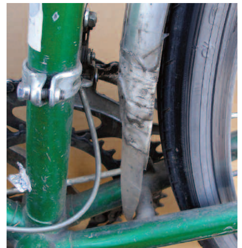
Problem: He "shifted" his fender rearward to give more coverage back there, but it left a gap on this other end.
