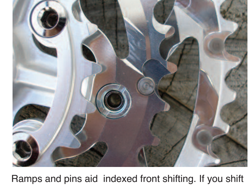
Ramps and pins aid indexed front shifting. If you shift friction in front like yotta, no feeeeeelable benefit.
